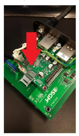
To get the PCB out of the casing, unscrew the 6 small screws in the front, and pull out the assembly.
